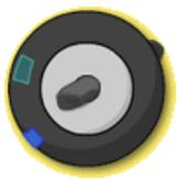
A **wheel and axle** is a large wheel attached to a smaller shaft (axle) which allows the wheel to rotate. The wheel and axle is the mechanism that makes a doorknob turn.
