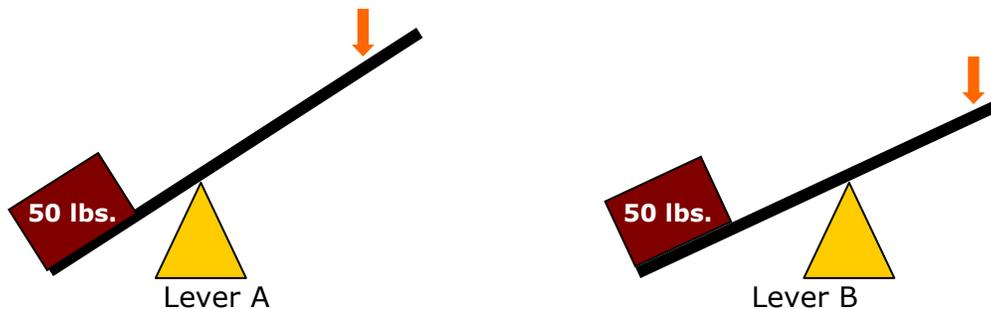
Which of the two levers require less force (in the direction indicated by the arrow) to lift the box?
