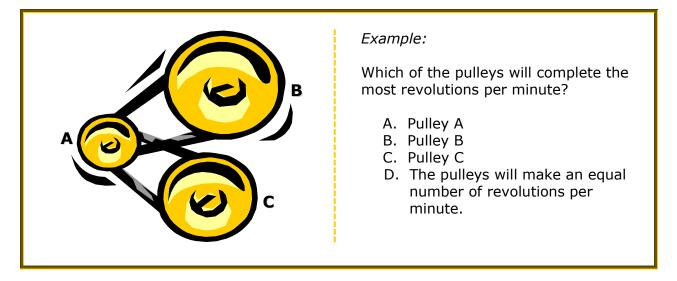
The answer is A. Notice that pulley A is the smallest of the three pulleys in the series. Because of its relative size, it has a shorter distance to travel to complete one revolution than do the larger pulleys. Thus, it can make more revolutions in the same amount of time. Another way to phrase this question would be to ask which pulley is moving fastest, in which case the same answer and supporting thought process is used.
