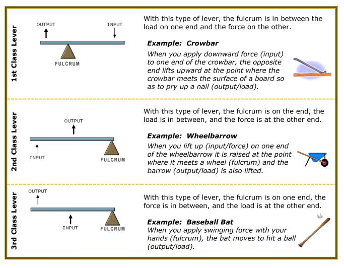
Most questions about levers focus on the 1st class of lever and are generally designed to test your understanding of the concepts of leverage and weight distribution. Considering this, the following *key facts* can be useful for answering the example questions on the next pages.
