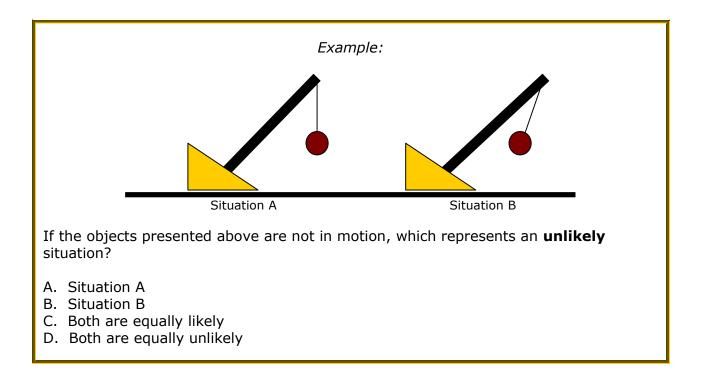
The answer is B. Because gravity always pulls objects downward, the ball at the end of the rope would be drawn straight down toward the ground. Hence, in the absence of some other force, such as a magnetic force, it is unlikely the ball would be suspended as presented in Situation B.
