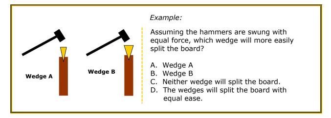
The answer is A. The farther the wedge can be driven into the board, the greater its ability to split the board. Wedge A can be driven into the board farther than Wedge B because it has a narrower angle that encounters less resistance from the board. As stated in the *key facts*, more force would be required to split the board with Wedge B because it meets more resistance at the point where it makes contact with the board, due to the wider angle of the wedge.
