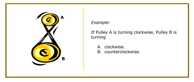
The answer is B. As stated in the *key facts* on page 7, whenever there is a twist in the belt between two pulleys, the pulleys rotate in opposite directions.
